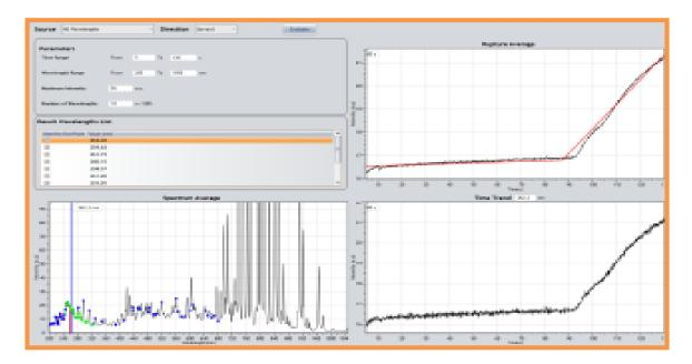
STEP3: The Endpoint simulation conducted by Rupture Intensity and the completed algorithm can be exported and built into Sigma-P. Endpoint is set on blue line when rupture intensity is the greatest, then over etch is applied.
