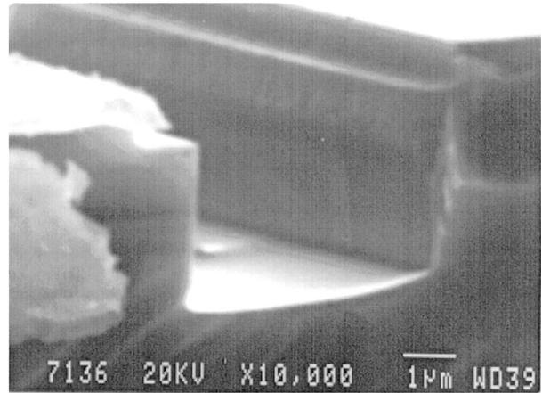
Fig. 1. SEM photograph of two adjacent devices formed by the optimized RIE conditions.
