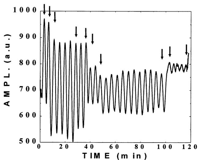
Fig. 2. Laser interferometry signal as a function of etching time for the laser structure of Table 1. The arrows denote heterointerfaces (see Table 1).
