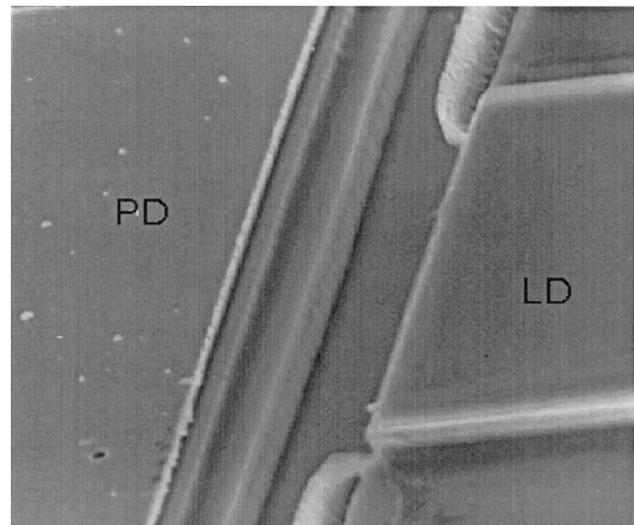
Fig. 3. SEM photograph of a laser diode (LD) next to a waveguide photodetector (PD) with RIE-edged mirrors. The distance between the mirrors is 5  $\mu\text{m}$ .
