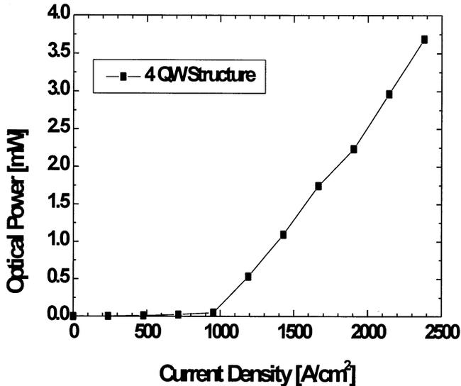
Fig. 4. Measured emitted power as a function of current density of a 4-QW laser diode, with RIE-etched mirrors.
